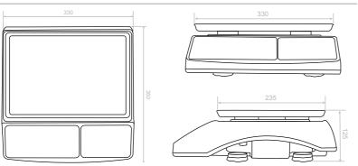
Fashionable design < Rugged ABS housing < Rechargeable 6V4Ah battery < Transparent dust-cover included < Aluminum load cell supporter < Four adjusting rubber feet < PC4 with rear display < PC4H with tower display < Fruit pan 310x225mm <
