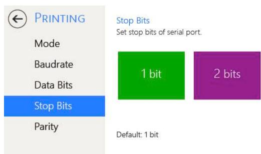
Stop bits (set stop bits of balance)
