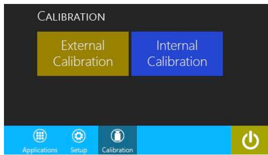
The balance will do the internal calibration, when finish, please press enter.
