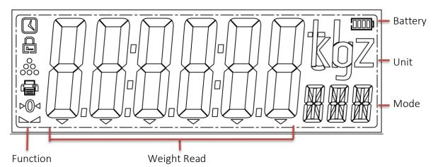
The backlight color can be set by the user, and also it allows to set different colors for checkweigh function (refer to F2.8 & F2.9)
