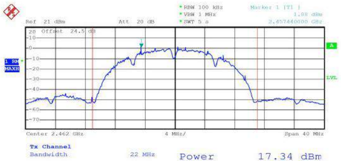
Figure 12 7104 Power Test Curve
