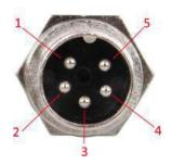
Pin1 - Excitation+ Pin2 - Excitation -Pin3 - Signal + Pin4 - Signal -Pin5 - GND for 6-wire load cells (short connect: +EXC and +SEN, -SEN and -EXC.)
