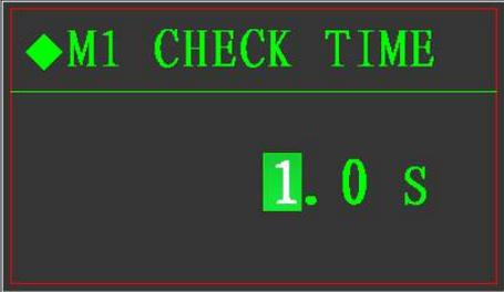
Choice: 0.0~9.9 seconds, the stabling time after batching finish of material 1
