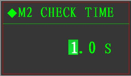
Choice: 0.0~9.9 seconds, the stabling time after batching finish of material 2
