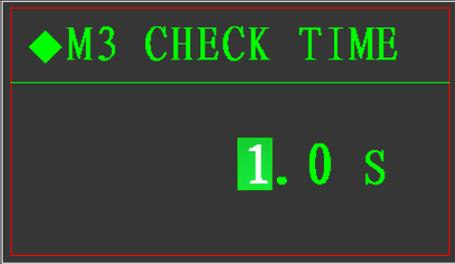
Choice: 0.0~9.9 seconds, the stabling time after batching finish of material 3
