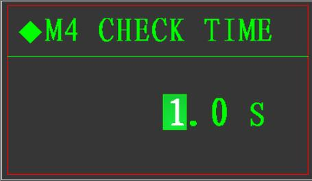
Choice: 0.0~9.9 seconds, the stabling time after batching finish of material 4
