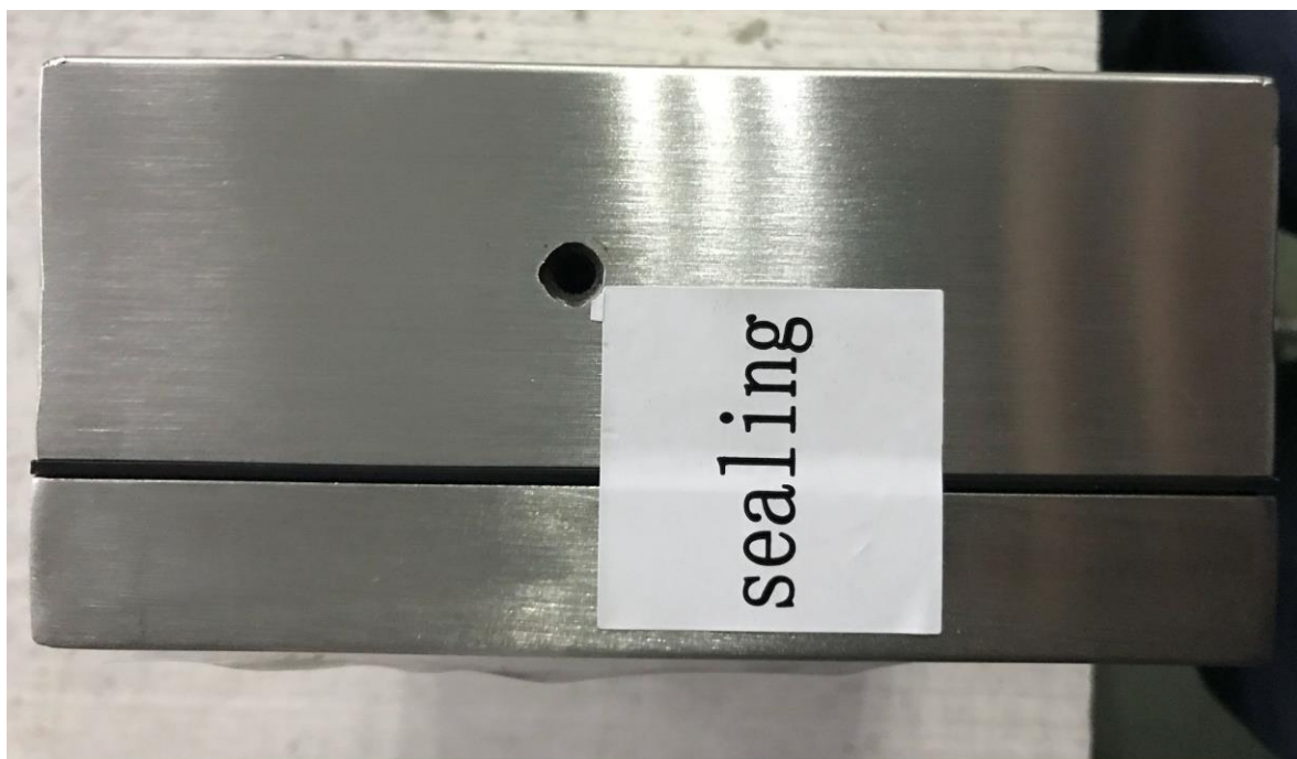
Figure 13 Sealing of indicator in stainless steel housing with stickers
