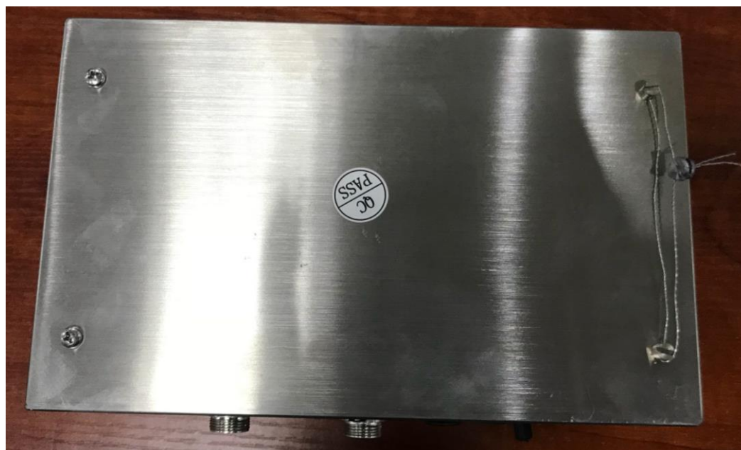
Figure 12 Sealing of indicator in stainless steel housing with wire and seal.
