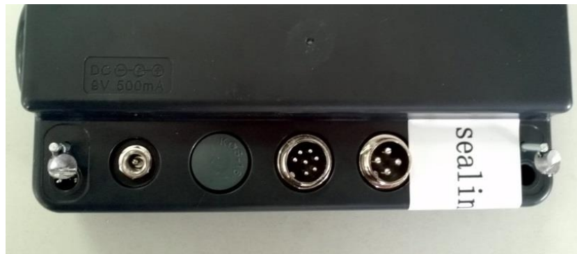
Figure 5 Sealing of X2 indicator
