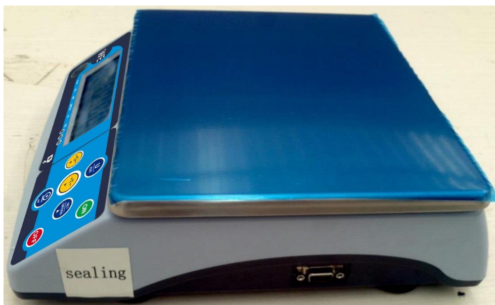
Figure 7 Sealing with stickers of PC1 / WE / CSQ scales.
